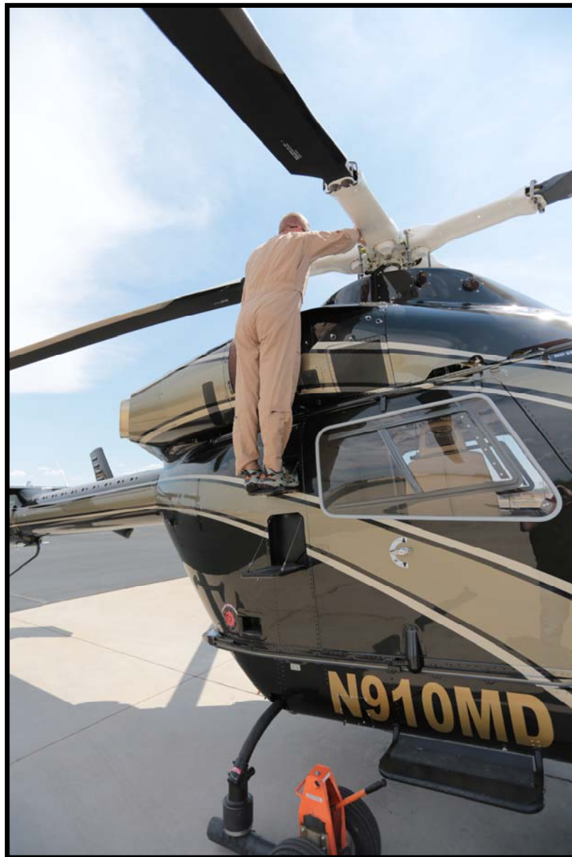
The MD 902 Explorer has Built-in Steps to Provide Access to the Engines and Main Rotor Head Without External Ground Support Equipment
